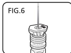
**15° Nozzle – Yellow:** This nozzle delivers a powerful 15 degree spray pattern for intense cleaning of small areas. This nozzle should only be used on areas and materials that can withstand high pressure.
