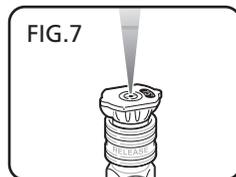
**25° Nozzle – Green:** This nozzle delivers a 25 degree spray pattern for intense cleaning of larger areas. This nozzle should only be used on areas that can withstand pressure from this nozzle.
