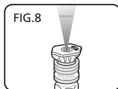
**40° Nozzle – White:** This nozzle delivers a 40 degree spray pattern and a less powerful stream of water. This nozzle can cover a wide area and should be used for most general cleaning jobs
