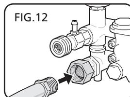
**NOTE:** The pressure washer requires a minimum of 20psi and a flow rate of 19L/m.
