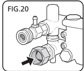
**WARNING: Do not operate pressure washer without screen filter in place. Impurities entering pressure pump can cause internal damage.**
