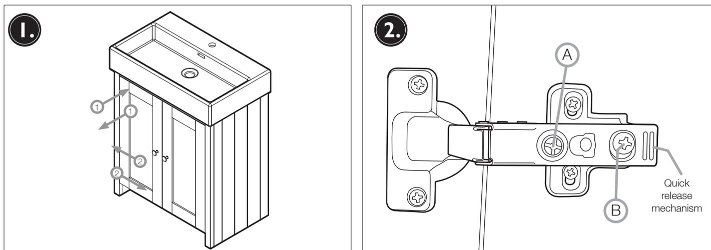
To make adjustment 1 tighten/loosen adjustment B.
