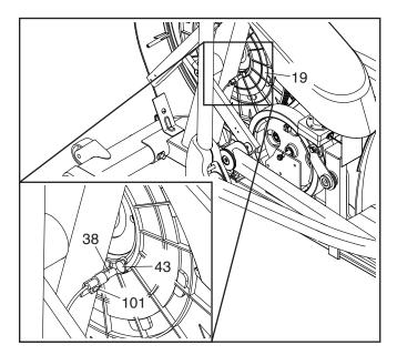
Slightly loosen the indicated M4 x 16mm Screw (101). Slide the Reed Switch (38) slightly closer to or away from the Magnet (43), and retighten the Screw.
