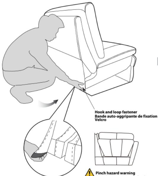
**5 Affix back cover to bottom of the frame using the built in hook and loop fastener strip.**
