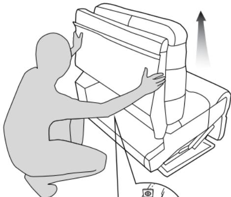
*Unlock metal locks, then lift the back firmly to remove.*
