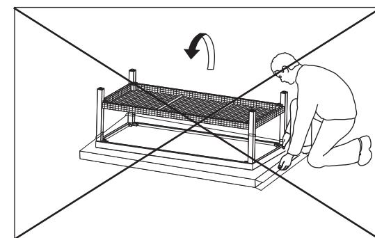
**⚠** Do not use any table leg as a pivot point to turn over the table.
