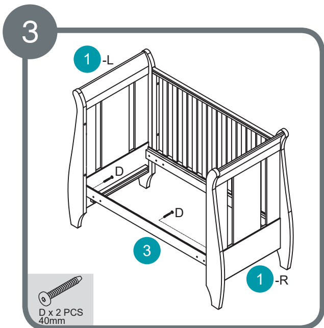
Assemble front mattress support bar using 2 x D bolts
