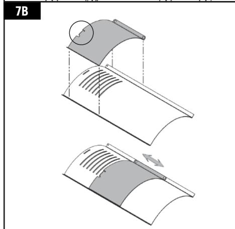
**NOTE: If the flame broiler main plate lays flat, on the base of the barrel, it is installed incorrectly. The flame broiler should set at an angle, with the left side sitting higher than the right.**
