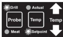
To adjust the SETPOINT temperature of the grill, press the **PROBE button** to indicate that the GRILL probe temperature is presently being displayed. Press the **TEMP button** to indicate that the SETPOINT temperature is selected, and press the UP or DOWN **Temperature Adjust Arrows**, adjusting by five degree increments, to your desired temperature.
