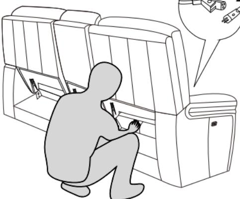
*Push down firmly on seat back to lock connectors.*
