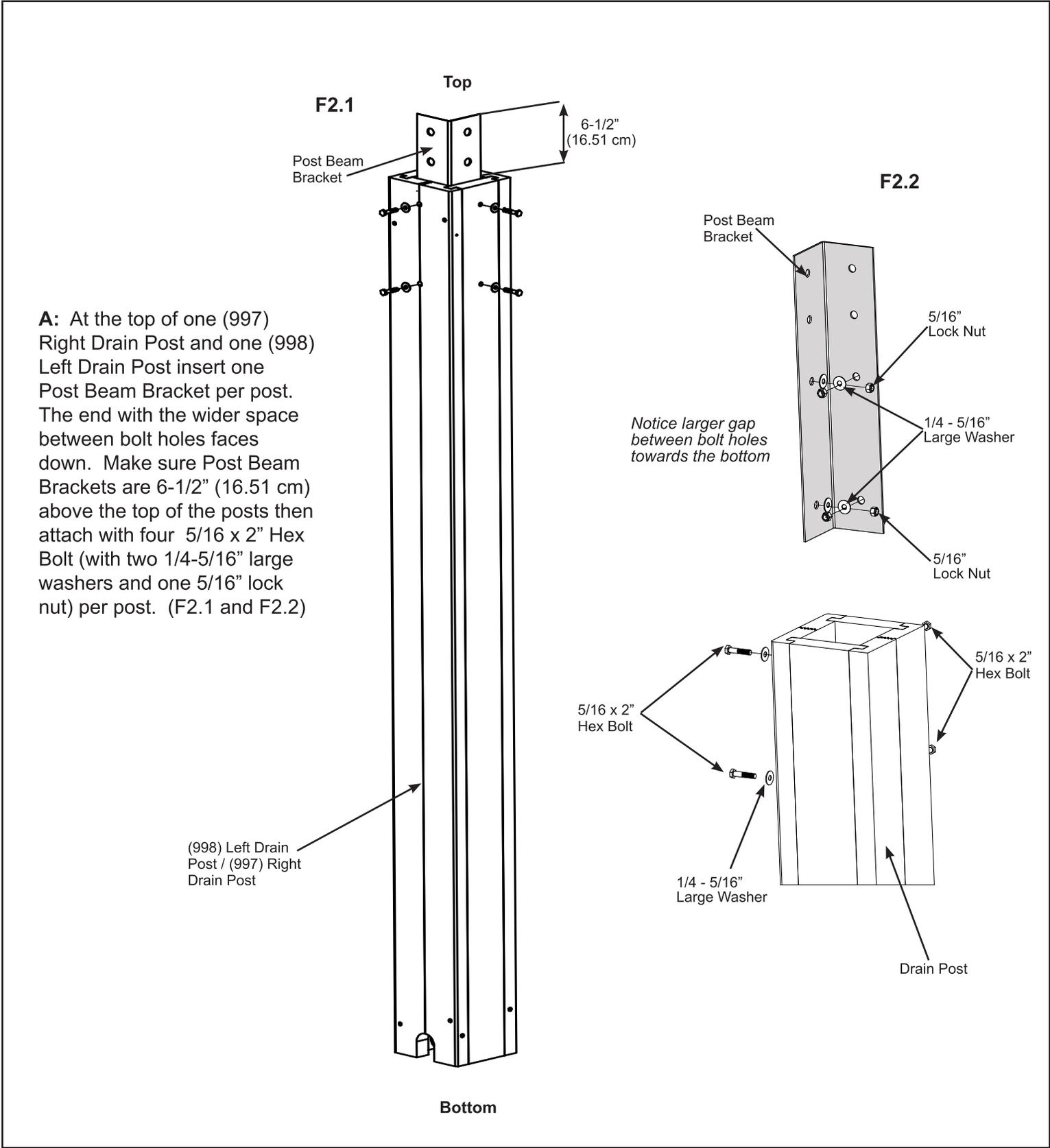
**A:** At the top of one (997) Right Drain Post and one (998) Left Drain Post insert one Post Beam Bracket per post. The end with the wider space between bolt holes faces down. Make sure Post Beam Brackets are 6-1/2" (16.51 cm) above the top of the posts then attach with four 5/16 x 2" Hex Bolt (with two 1/4-5/16" large washers and one 5/16" lock nut) per post. (F2.1 and F2.2)
