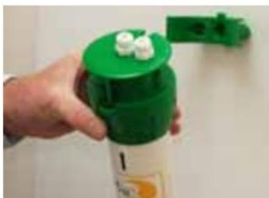
5. Standard 3/8"- 1/4" push fit elbow 90° fittings are supplied with the product. Fit the push fit fittings to the upstanding port spigots ensuring that the blue 'U clip' is in place – this is required for push fit removal on cartridge change. Use the white spanner to assist pushing it into place if need be.
