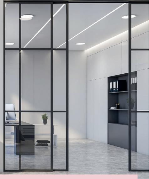
Our sliding doors operate on an aluminium track, positioned at the top of the doors. This ensures that the floor level remains flush for ease of access between rooms. Rather than opening into a room, you can choose whether your sliding doors will gently glide parallel to the internal wall, where they will sit neatly whilst open, or by creating a purpose-built cavity, the doors give the illusion of disappearing, to create a 'pocket sliding door' system.
