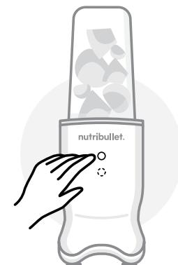
7 Twist the **Cup** clockwise onto the **Motor Base** to lock it into place. (A "click" signals that the **Cup** is locked.) This will illuminate the **Control Panel**.
