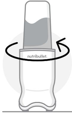
9 Twist the **Cup** counterclockwise to unlock and remove it from the **Motor Base**. You will hear a "click" when the **Cup** unlocks. Enjoy!
