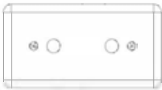
V01 LATCH BLOCK - W4L19102 (x1) 1 1/4"x1 1/4"x2 3/8" (32x32x60)
