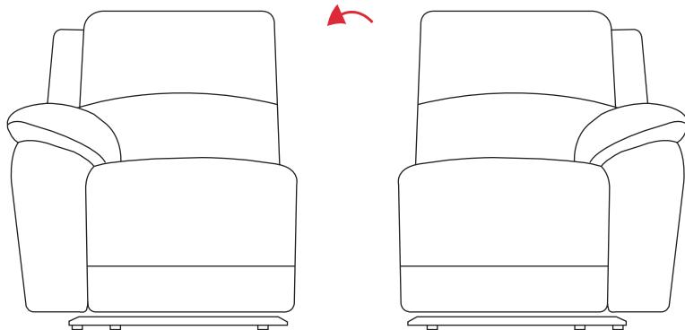
Ensure both pins are securely located into the slots.
