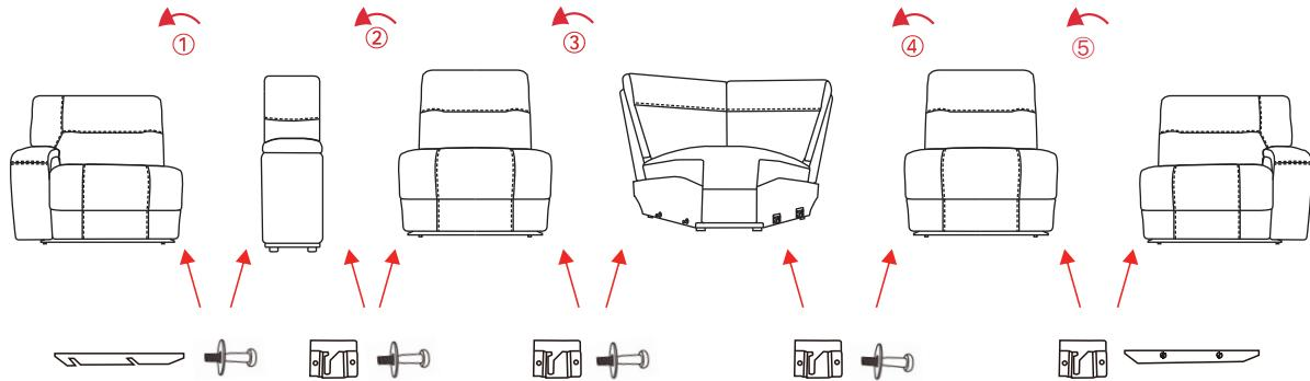
Ensure both pins are securely located into the slots.
