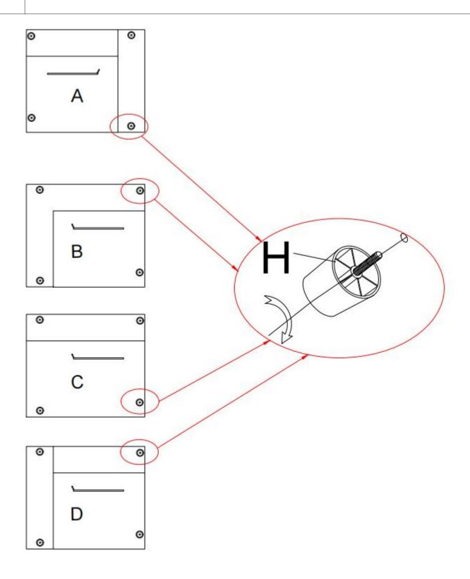
Assemble the matching plastic feet H onto the bottoms of A, B, C, and D, and fully tighten them. Place the left A, B, C, and D together and lock them in sequence using the vise grip kit. Arrange the foot pad E according to actual requirements, place the backrest in the direction indicated by the arrow, and align and fasten the two ends of the zipper together.
