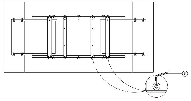
In case the extension leaves are not operating correctly please note these can be adjusted. loosen the allan bolts on the underside of the frame as indicated in the image. Adjust the metal plates that connect the main frame. tighten once adjusted.
