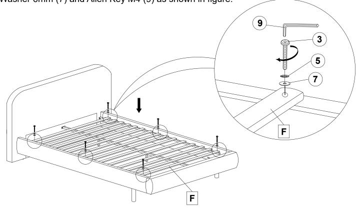
**Step 7**Assemble Slat (F) using CSK M4 x 30mm (8) with Screwdriver as shown in figure.
