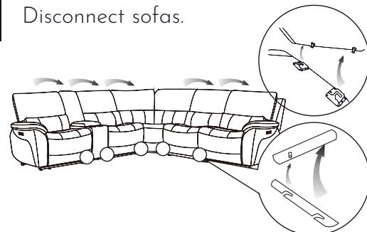
**4** Remove hook and loop fastener. Disconnect cable.
