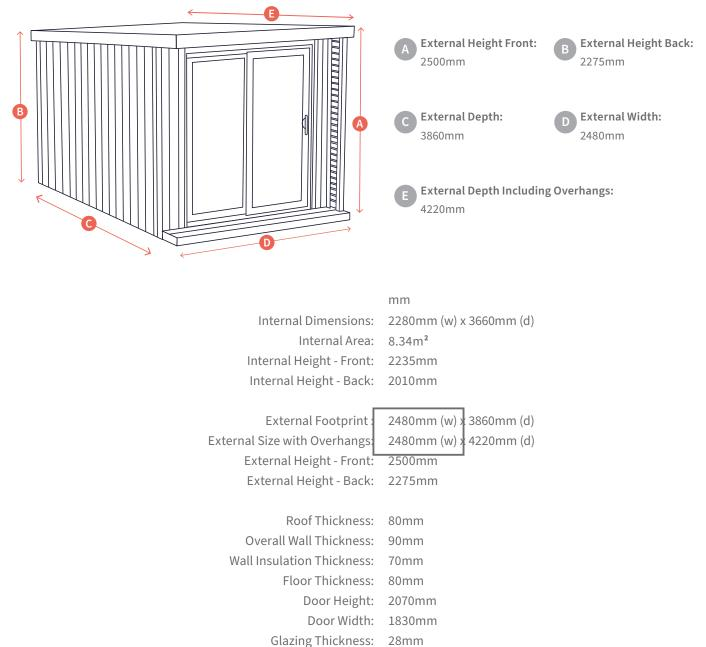
All buildings have a 300mm front overhang on the roof, and a 110mm gutter at the rear.
