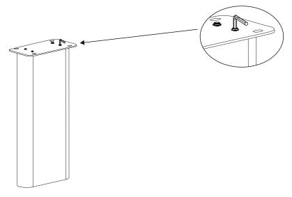
**IMPORTANT:** Hand tighten only to avoid damage to the legs.
