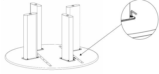
**IMPORTANT:** Hand tighten only to avoid damage to the legs.
