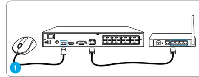
Connect the NVR (LAN port) to your router with an Ethernet cable. Next, connect the mouse to the USB port of the NVR.
