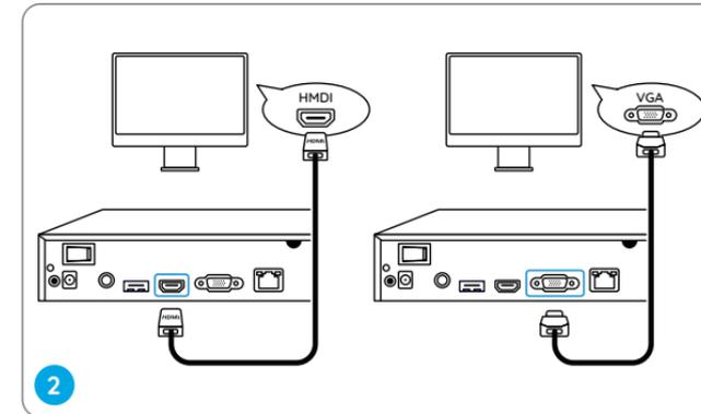
Connect the NVR to the monitor with a VGA or HDMI cable.
