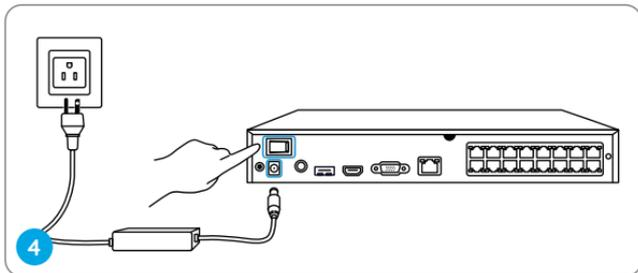
Connect the NVR to a power outlet and turn on power switch.
