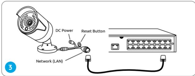
Connect cameras to PoE ports on the NVR.
