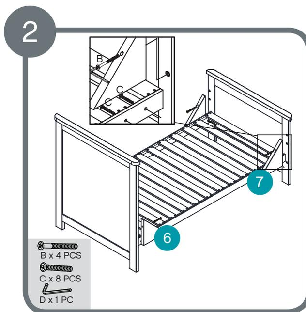
Assemble triangle braces support using 4 x B bolts and 8 x C bolts
