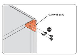
NOTE: CAREFULLY ROTATE THE BOX ONTO ITS SIDE; WE RECOMMEND USING A SCRATCH-RESISTANT SURFACE TO PROTECT THE PAINTWORK. LOCATE AND SECURE FEET 0249-16 AT THE LOCATIONS INDICATED ABOVE.
