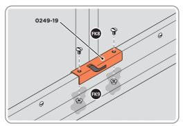
NOTE: MAKE SURE THE CATCH PLATE IS IN THE CORRECT ORIENTATION. LOCATE AND SECURE PLATE 0249-19, AT LOCATIONS INDICATED ABOVE.
