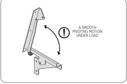
**NOTE:** AFTER TIGHTENING THE NUT & BOLT, ENSURE THE HINGE OPERATES SMOOTHLY WHILST MAINTAINING RESISTANCE ON THE FRICTION WASHER.
