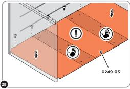
ONCE LOWERED INTO POSITION, LOOSELY ATTACH AT (x6) LOCATIONS. NOTE: IF APPLYING BODY WEIGHT TO FLOOR, ONLY USE AREAS INDICATED ABOVE, WHICH HAVE EXTRA STRENGTH AND SUPPORT.
