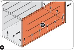
$\mbox{NOTE}:$  INWARD ADJUSTMENT OF SIDE PANELS REQUIRED, SECURE ALL THREE PANELS TO BASE, AT LOCATIONS INDICATED ABOVE .
