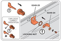
WITH THE LID IN THE UPSIDE DOWN POSITION, SECURE LOCK BACKING PLATE 0249-25 AND CAM LOCK ASSEMBLY TO LID AS SHOWN ABOVE. NOTE: M22 SOCKET WILL BE REQUIRED FOR LOCKING NUT.
