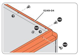
NOTE: MAKE SURE THE LOCK CUTAWAY IS IN THE CORRECT ORIENTATION. LOCATE AND SECURE FRAME 0249-04, AT LOCATIONS INDICATED ABOVE.
