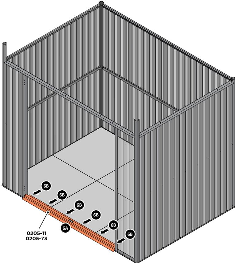
**IMPORTANT:** ONCE FLOOR PANELS ARE POSITIONED CORRECTLY, WE STRONGLY RECOMMEND YOU SECURE THE FLOORING TO THE BASE. FOLLOWING INSTRUCTIONS ON PAGE 7.
