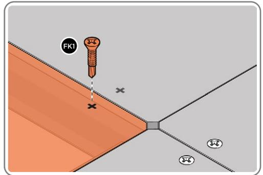
USE TEMPLATE TO SECURE FIXING SCREW FK1 TO EACH FLOOR PANEL MARKED.
