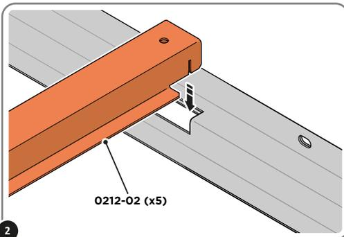
2 SLOT EACH FLOOR BRACE 0212-02 INTO POSITION AS SHOWN ABOVE.
