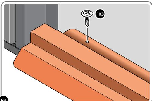
**6B** SECURE DOOR STRIP ONTO FLOOR PANELS AT x6 LOCATION INDICATED. PLEASE NOTE: THE FIXING USED IS A SELF DRILLING COMPONENT.
