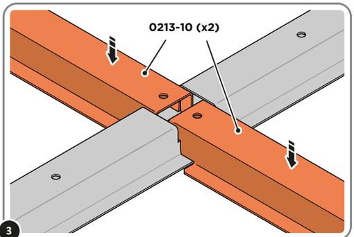
3 SLOT EACH FLOOR BRACE 0213-10 INTO POSITION AS SHOWN ABOVE. PLEASE NOTE: ENSURE TOP OF FLOOR BRACE IS LEVEL WITH TOP OF FLOOR RAIL
