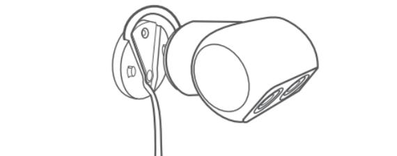
5. Slide the camera onto the mounting plate and make sure it is attached securely.
