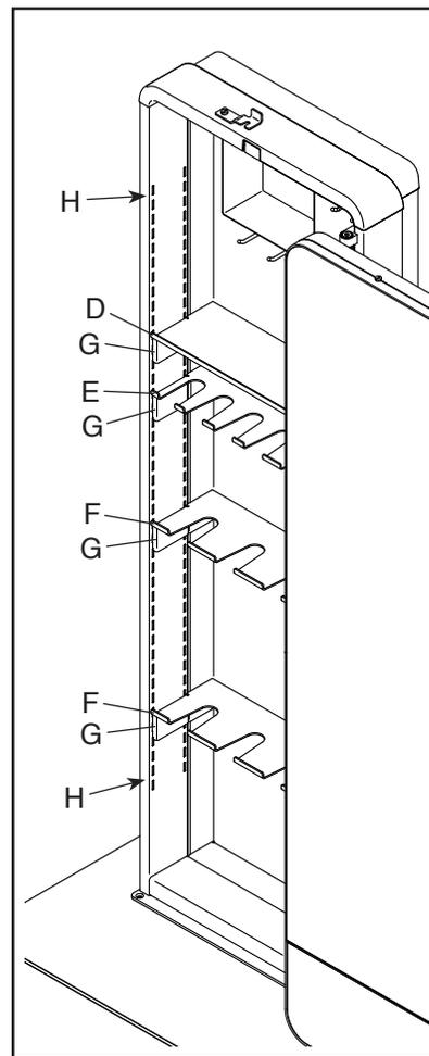
Then, press a shelf (D) or a rack (E, F) firmly into place over the hangers (G); it may be helpful to use a rubber mallet. Orient a shelf so that the tabs face downward and the lip faces upward at the front; orient a slotted shelf so that the slots face outward and the lip faces upward at the front.
