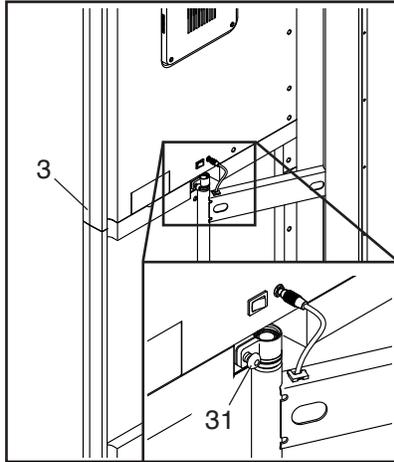
If the **hinge** does not move easily, or if the hinge moves too freely, the lower bracket in the cabinet needs to be adjusted.
