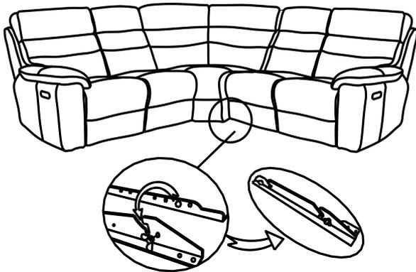
Lift up the right end sofa and join the brackets firmly onto corner sofa as above picture shown.
