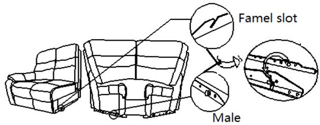
Lift up the corner sofa and join the brackets firmly onto left end sofa as above picture shown.
