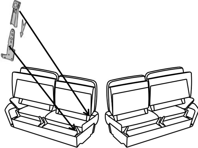
With the help of an assistant, join the back rest assembly to the base by locating the female fixing brackets on the male brackets as shown, and push down firmly into position;
