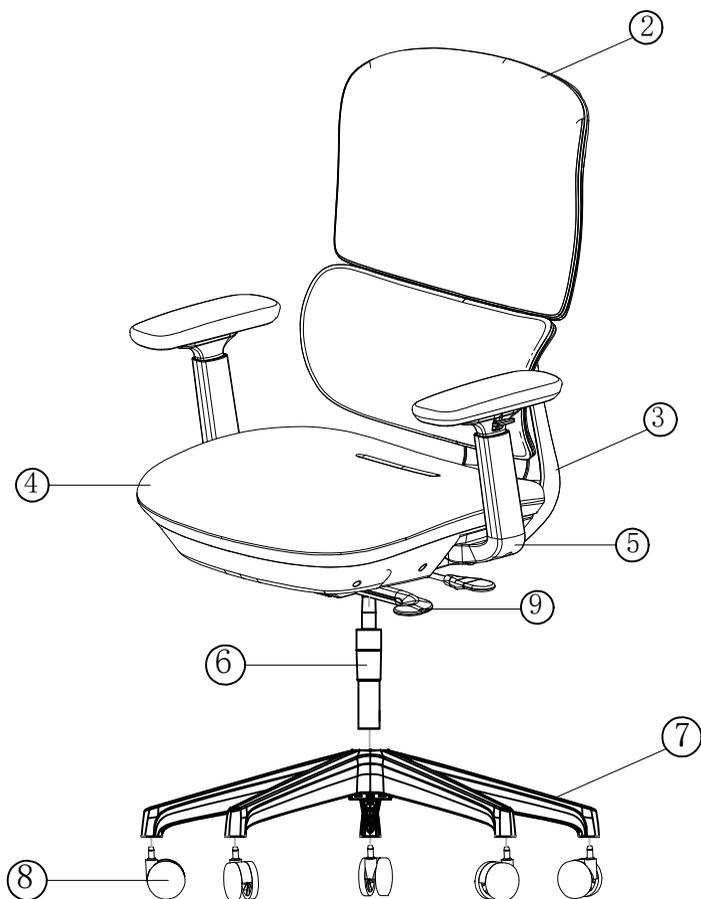
1. First loosen two screws pre installed on the headrest, and then use hex half-round-head screws to fix the headrest.
