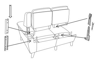
Align the backrest and the armrest on the back as shown in the picture, and align them downwards tightly
