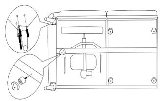
Align the plastic feet with the holes and tighten them clockwise; place the wooden feet on the four corners of the bottom of the sofa, and use the screws to align the holes and tighten
