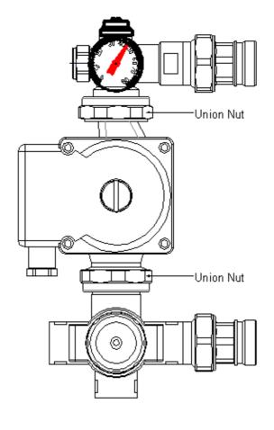
The valve works at lower temperatures than radiator systems, with temperatures between  $35^{\circ}$ C to  $65^{\circ}$ C depending upon the construction of the floor. The blending valve is the heart of the control system with hot water from the boiler mixed to supply water at the correct temperature back to the underfloor pipework. The supply temperature of the water can be adjusted to suit the construction of the floor.
