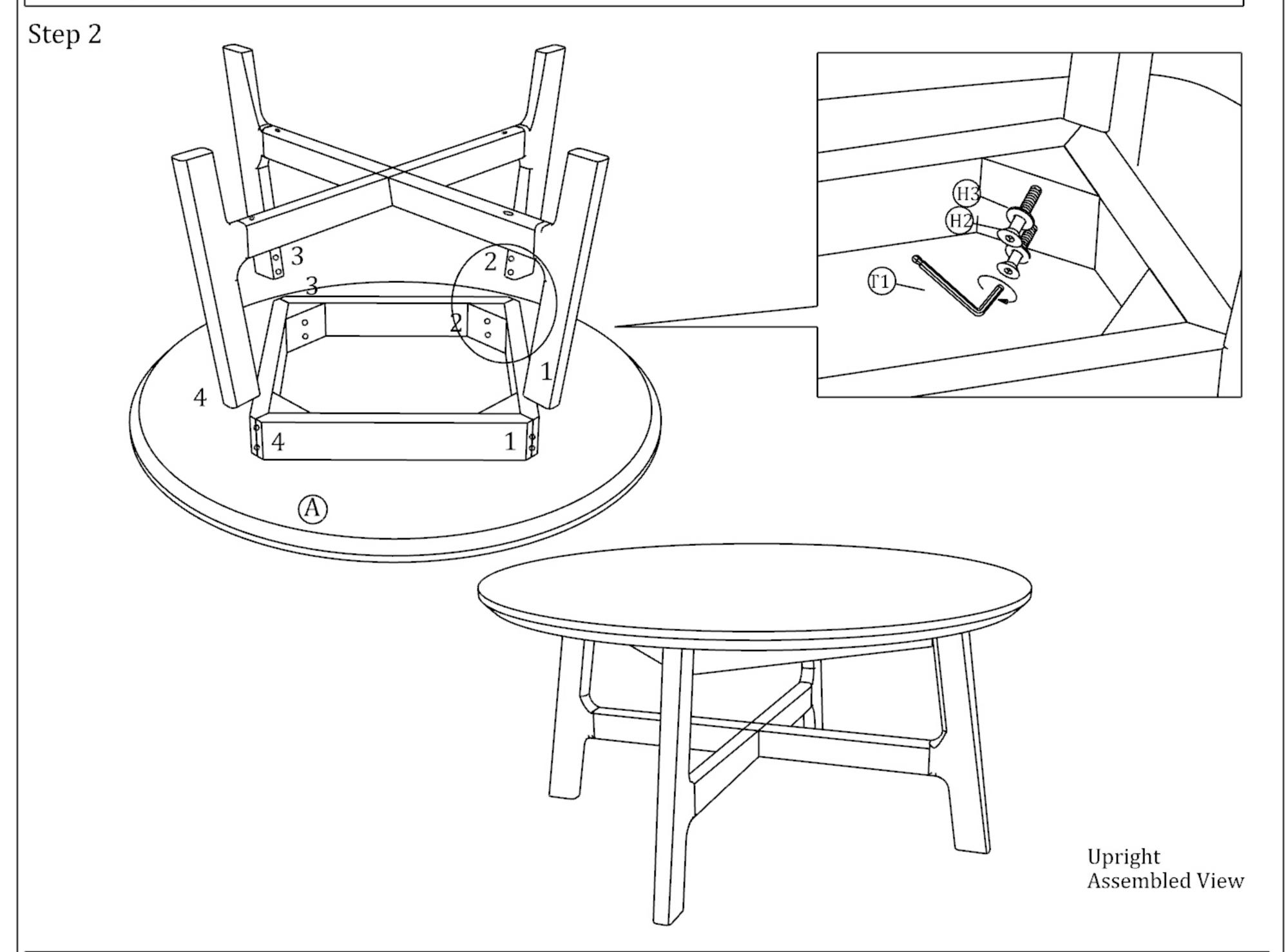
Align pre-assembled leg frame (B+C) onto Table Top (A) matching the markings - 1 to 1, 2 to 2...etc. Secure the connections with Large Allen Bolt (H2) and tighten it with Allen Key (T1). Repeat the step to secure all tightly. Turn the piece upright. Product is ready to use.
