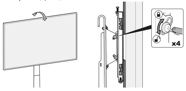
Adjust screws to achieve perfect tilt resistance if required. You can also lock the tilt if required.
