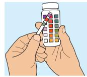
**Warning:** Very high chlorine levels (above 15mg/l) can bleach indicator pads on test strips.
