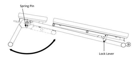
Pull spring to unfold or fold leg. Make sure hands are clear of pivot area. Make sire spring pin is fully engaged in locking holes after each adjustment.
