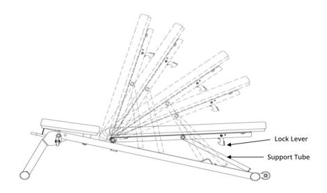
Swivel lock lever under pad to release back pad. Raise the head end of the pad so the free end of the suport tube slips into a slot for a desired position. Before use, make sure the support tube is secure in a slot.
