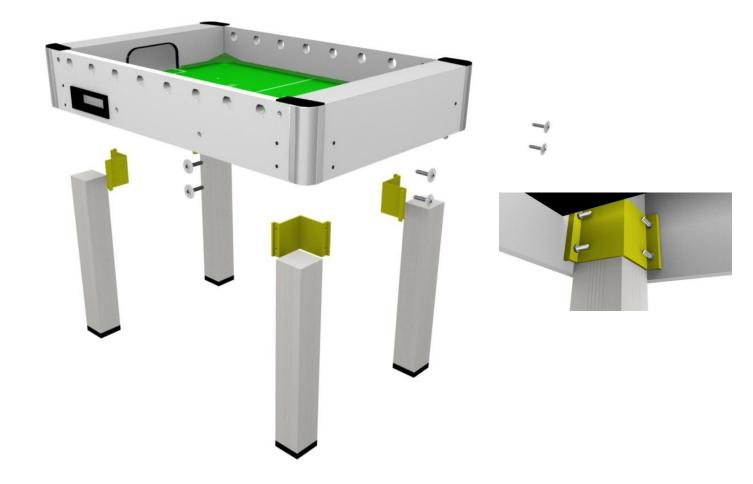
Set the L shaped bracket internally the table boby and insert the aluminium leg inside the L bracket. To block them, insert from the external of the body the screws 8x45 with washer 8x32 and tighten them up with the allen screw
