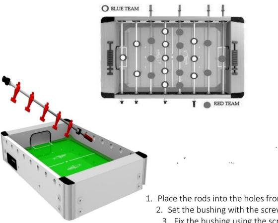
1. Place the rods into the holes from the handles side. 2. Set the bushing with the screw holes upwards 3. Fix the bushing using the screw (5x20 mm)
