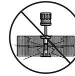
This icon warns you to not over tighten your bolts. This is to prevent structural damage and also splintering your wood.
