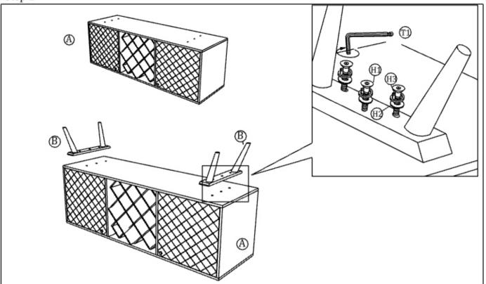
Place Sideboard Body (A) upside down on a non-damaging padded surface. Align Leg (B) with Sideboard Body (A) as shown above. Insert Allen Bolt (H1), Washer (H2) and Spring Washer (H3) and tighten it with Allen Key (T1). Follow the same process to attach other Legs (B). Fully tighten all connections with Allen key (T1). Turn the piece in upright position.
