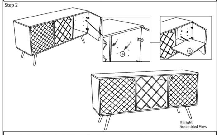
Open the door and fix the Shelf Pin (H4) in the desired holes,and place The Wood Shelf (C) on Shelf Pin as shown above in the drawing. Follow the same process to place the other shelf. Product is ready to use.
