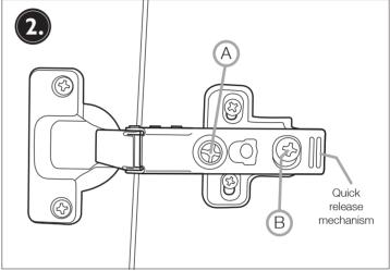
To make adjustment 1 tighten/loosen adjustment B. To make adjustment 2 simply turn screw A.
