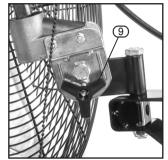
Select the angle required using the square body coach bolt and lock in place using the plastic head thumb bolt (9).
