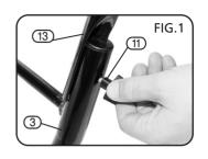
Attach the cable tidy by slotting into the holes on top of the nozzle panel.
