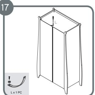
Assemble antl falling hardware L.
