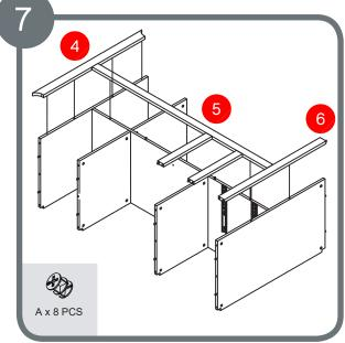
Assemble locking nuts 3 x A.
