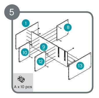
Assemble locking nuts 10 x A.
