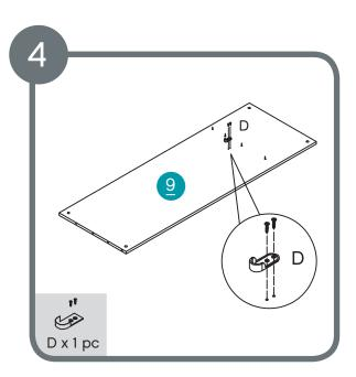
Screw hanging rail support D x 1 into divider.
