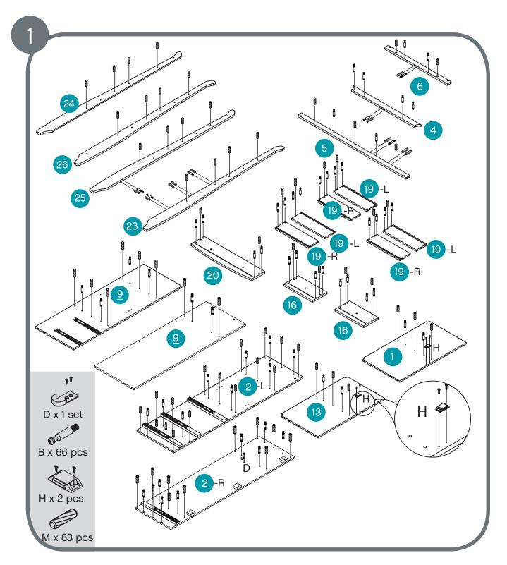
Assemble metal dowels B x 66 and wooden dowels M x 83. Assemble magnetic catches H x 2 to top and hanging rail support D x 1 to side.
