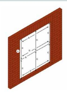
**NB:** Before the survey, ensure your opening is within 50mm of the maximum width you have chosen.
