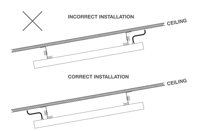
The supply cable must be at the lower end of the heater if the heater is installed at an angle or vertically.
