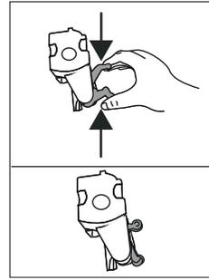
9. Once inserted, make sure the two coloured buttons have snapped out;
