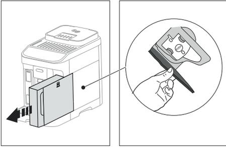
4. Press the two coloured release buttons inwards, at the same time pulling the infuser outwards;
