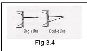
For pulls over 70% rated line pull, we recommend the use of the snatch block/pulley block to double line the wire rope. Fig 3.4
