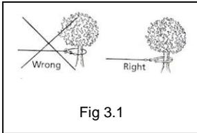
Locate a suitable anchor such as a strong tree trunk or boulder.
