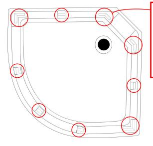
Apply RubberGum to raised sections of the tray and remove backing paper.
