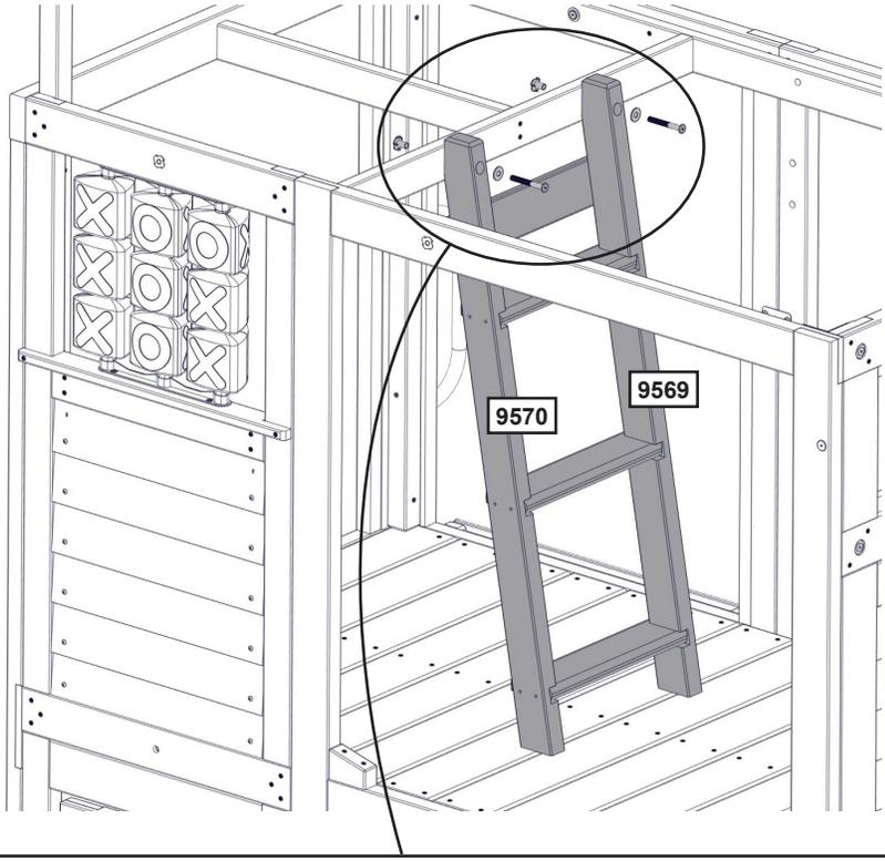
**Assemble T-Nuts first with hammer!**
