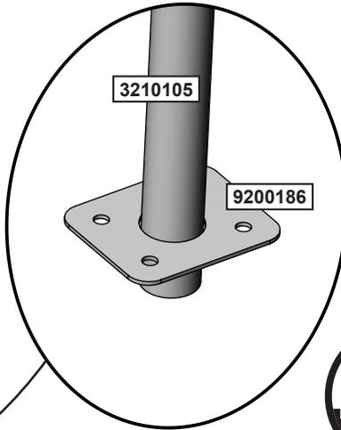
Make sure the Fireman Pole is straight and that the bottom of the pole is inserted into the ground as needed.
