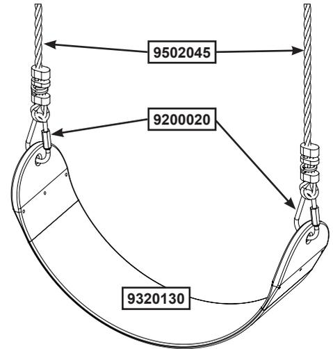
**Caution:** Threaded Quick Links must be installed with the gate completely down covering the threads and tighten as instructed.
