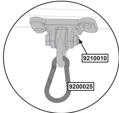
**Caution:** The Spring Loaded Quick Link must be attached to the Heavy Duty Swing Hanger in the closed position.
