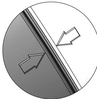
Align each elbow using the molded arrows.
