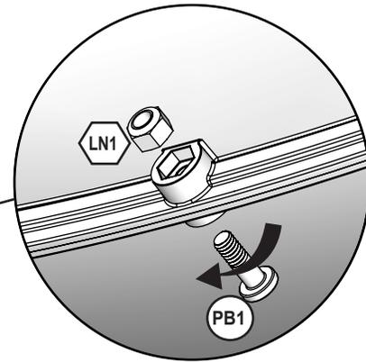
Remove PB1 (1/4 x 3/4" Pan Bolt), The bolt (PB1) will no longer be needed, but keep the lock nut (LN1)
