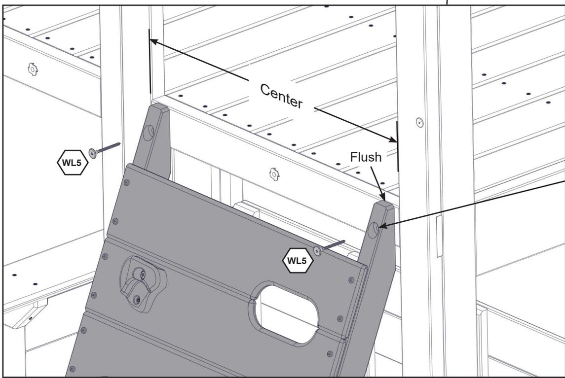
**Pre-drill each hole using a 1/8" drill bit for WL5.**
