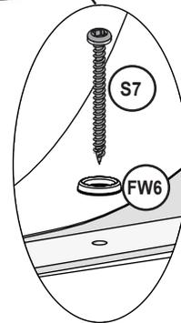
Pre-drill each S7 hole using a 1/8" drill bit. Making sure the pre-drilled holes are a minimum of 1" deep.
