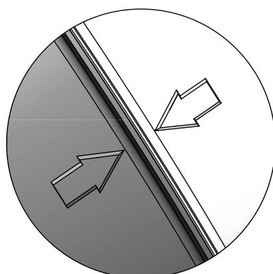
Align each elbow using the molded arrows.
