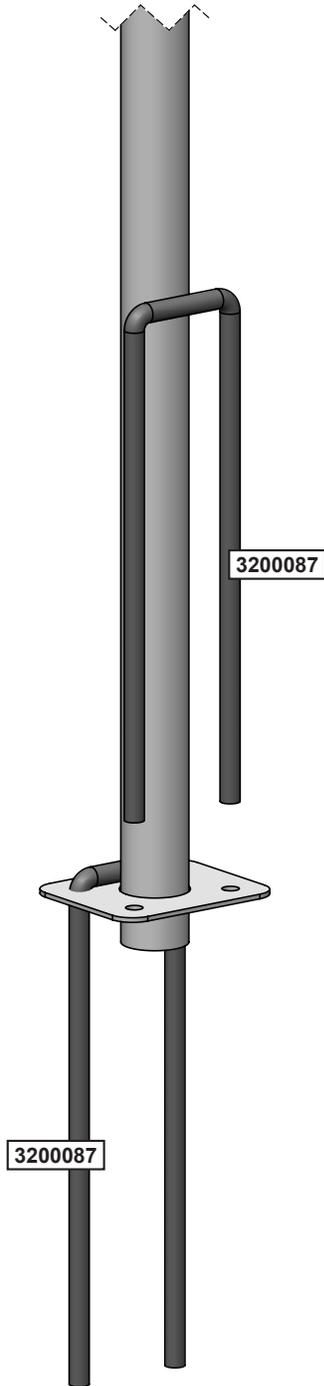
pole is to be 1-1/4" into the ground when installed
