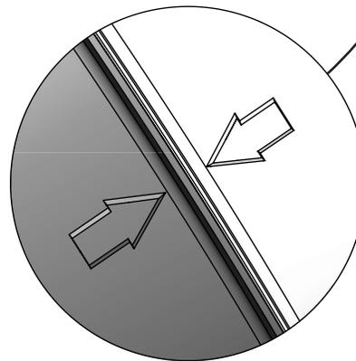
**Align each elbow using the molded arrows.**
