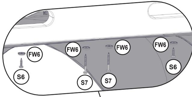
Pre-drill each S7 hole using a 1/8" drill bit. Making sure the pre-drilled holes are a minimum of 1" deep.
