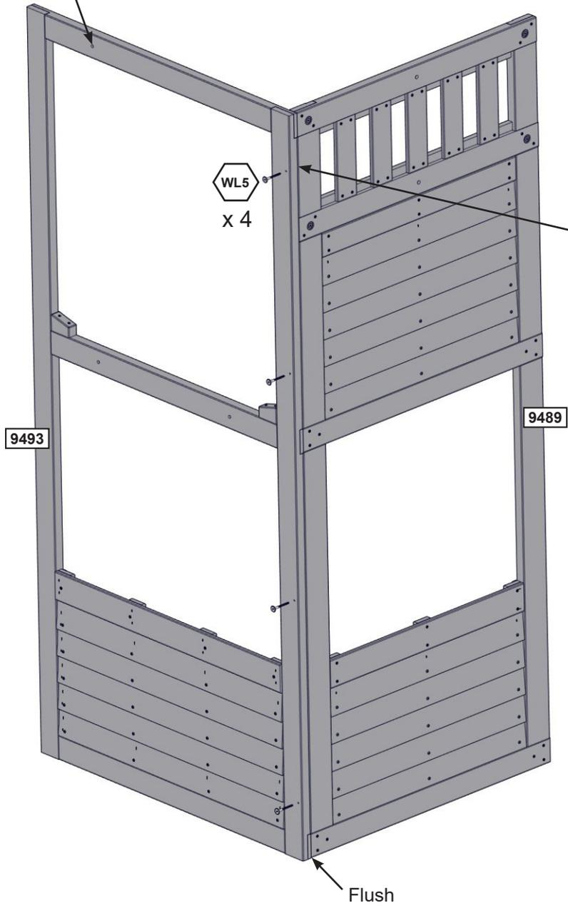
Pre-drill each hole using a 1/8" drill bit for WL5.
