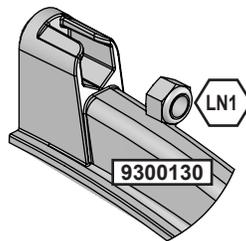
**Note: For ease of assembly bottom set of clamp rings can be rotated 90 degrees to install bolts.**
