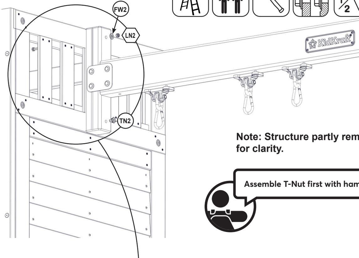
Assemble T-Nut first with hammer.
