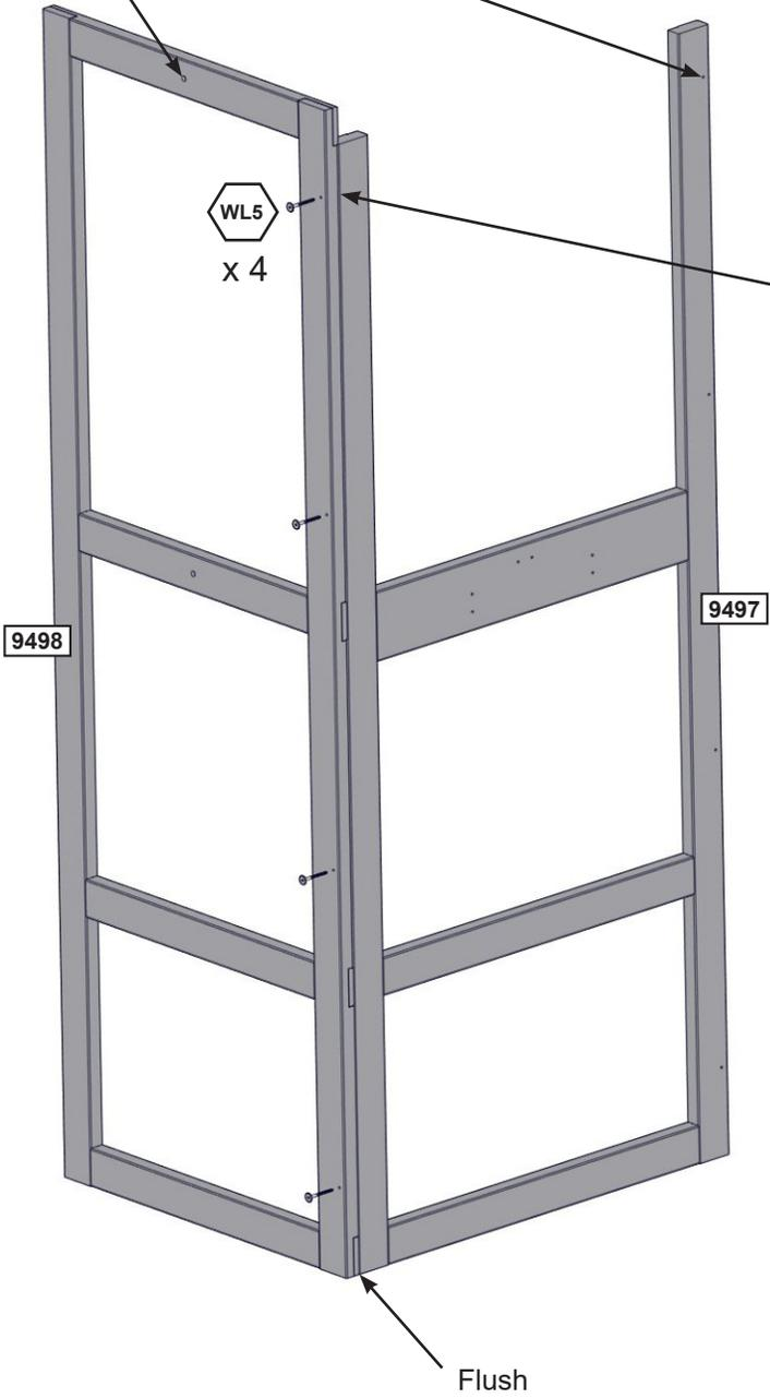
Pre-drill each hole using a 1/8" drill bit for WL5.
