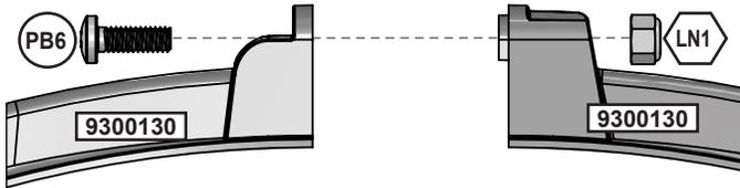
After the clamp rings are attached to the elbows, fasten them end to end with two pan bolts and lock nuts
