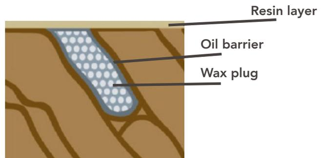
of the cells. As the solvent evaporates, the oil thickens, and the wax hardens but remains flexible. The resin settles on top of the cells and dries hard. When a second or third coat is applied the solvent reactivates the wax, oil, and resin and allows the additional coats to blend with previous coats. The more coats applied the deeper the finish penetrates into the pores.
