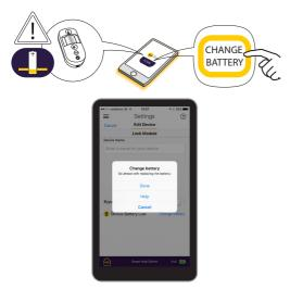
When a device first shows the low battery signal in the app, it has enough capacity to operate for approx 1 month before complete exhaustion.
